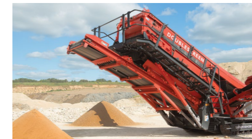
Three sided walkway around main conveyor
