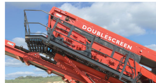
Patented double deck Doublescreen technology
