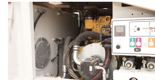
Efficient hydraulic system and low RPM for fuel economy
