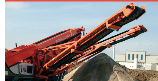
Hydraulic slew and raise / lower facility
