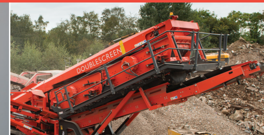
Hydraulically folding walkways for ease of maintenance
