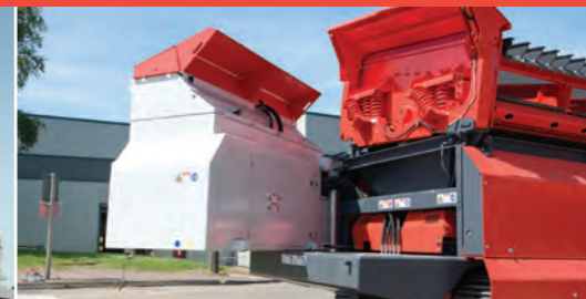
Hydraulically opening powerpack for ease of maintenance
