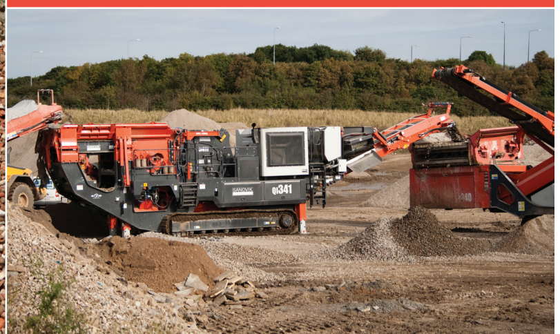
Featuring Sandvik's unique CI411 Prisec™ impact chamber (5 patents pending). The Prisec™ concept enables one base crusher to be configured as either a Primary or Secondary chamber whilst maintaining optimum crushing geometry.
