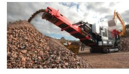
Long main conveyor for massive stockpiling
