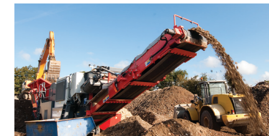
Long main conveyor for massive stockpiling
