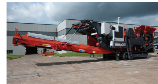
Hydraulic raise / lower facility on main conveyor for increased clearance
