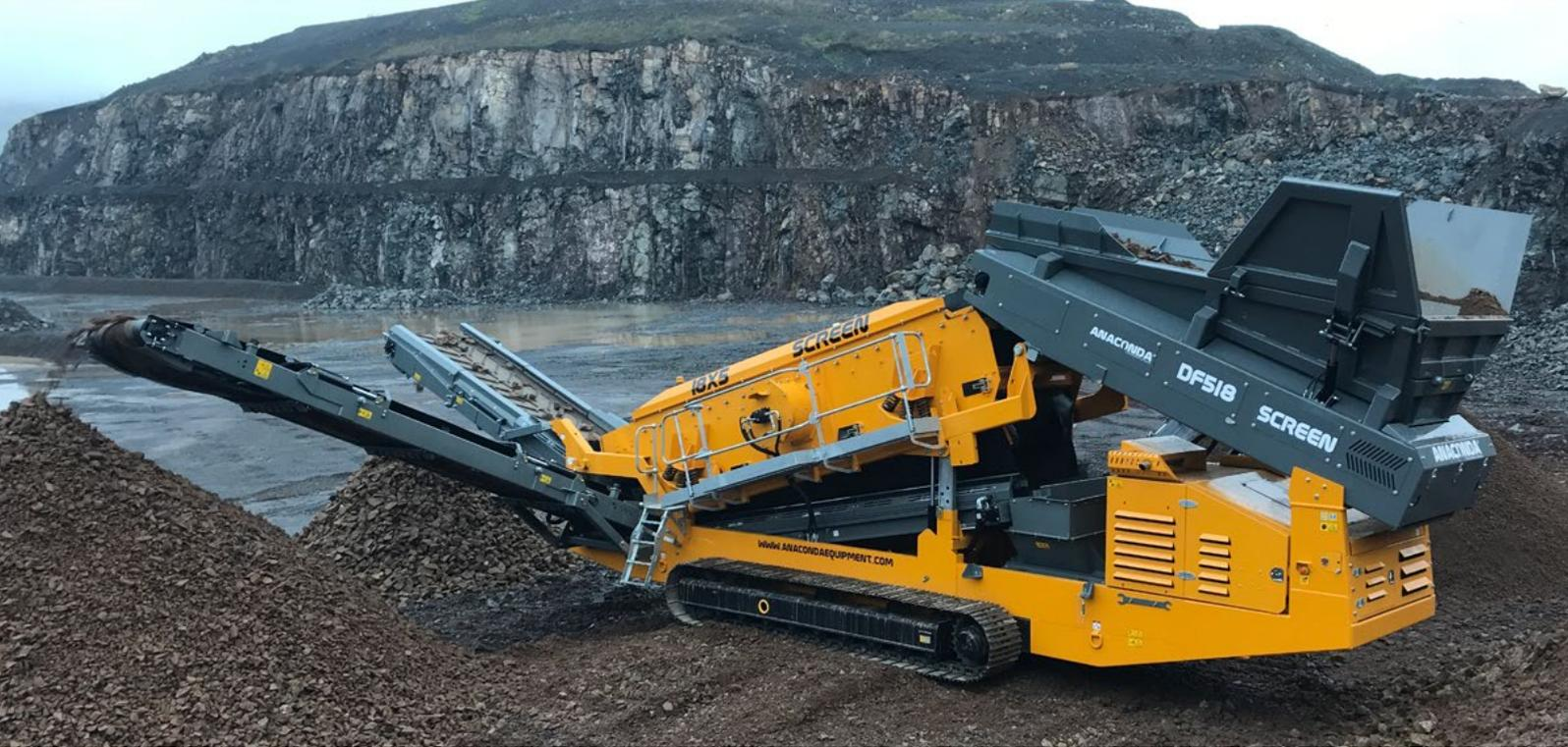
The Anaconda **DF** Range of Mobile Tracked Scalping Screens are Heavy Duty Screens that has been developed specifically to suit a variety of applications.
