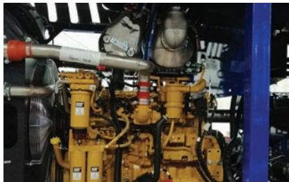
Tier 4 Final / Stage 5 - CATERPILLAR C9.3B 310Kw (420HP)
