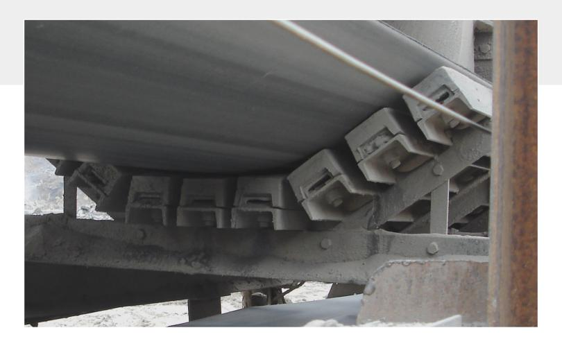
Douglas Impact Beds are engineered to protect the conveyor belt at key transfer point areas. They help to keep material on the belt where it belongs. Impact beds help to absorb shock loads and support the full width of the conveyor belt. They help to eliminate the cost of idler maintenance and failure. No more bent idler shafts and frames, or worn out rollers to replace.
