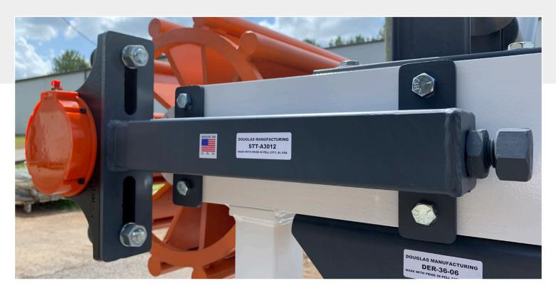
Available in seven different styles to suit your specific needs: Slide Tube™, Top Angle, Center Pull, Heavy Duty Top Mount, Light Duty Top Mount, Wide Slot Side Mount and Scissors Pivot Gravity Take-Up Assembly. Douglas take-up frames utilize many common styles of bearings from most major bearing manufacturers (bearings are provided separately).
