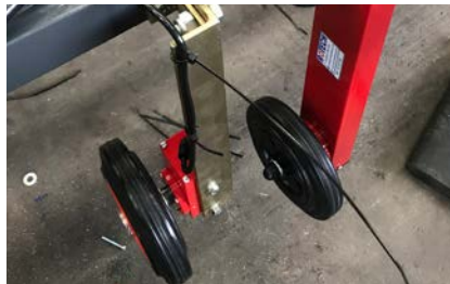
Belt Scale - fitted to collection conveyor.
