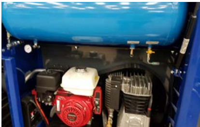
Air Compressor - multiple air line inlet-ports provided.
