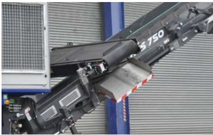
Overband Magnet - Hydraulic height adjustable, twin pole magnet.
