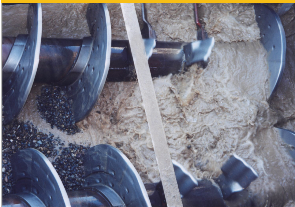
A look inside at the paddles and shaft of a coarse material screw washer.
