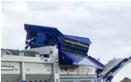
Twin Deck Vibrating Grid - Available with remote tipping function
