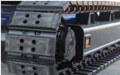
Rubber Track Pads - perfect for operating on hard surfaces
