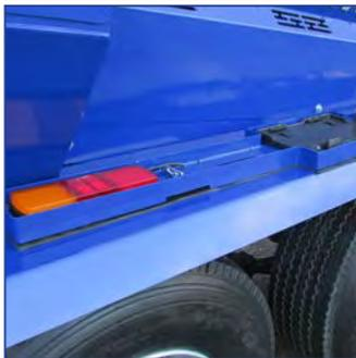
Lighting boards available for road towing. Must specify voltage
