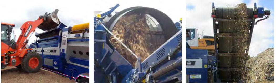
The TR622 Trommel combines high production rates with ease of use in a robust, portable and versatile screening plant that is ideal for applications such as top soil, recycling, composting and is proven in construction and demolition waste.
