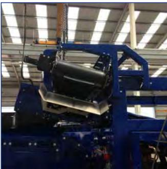
Overband magnet fitted to collection conveyor to extract ferrous metal
