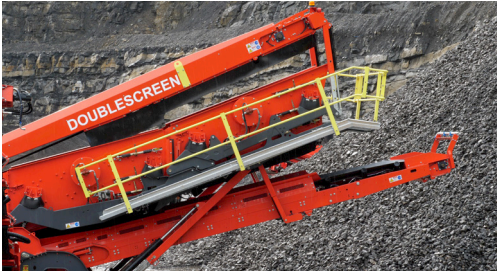
Triple deck Doublescreen with independant screen angle adjustment and screen separation, patent pending
