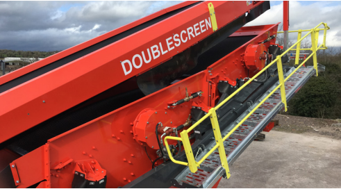
Hydraulically folding walkways for ease of maintenance
