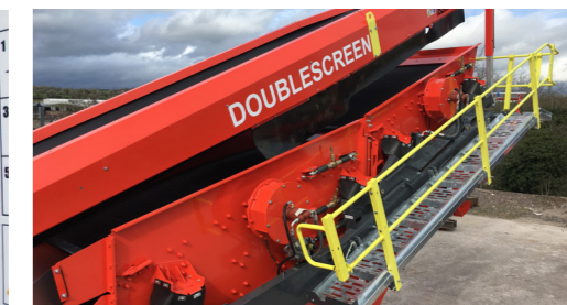
Hydraulically folding walkways for ease of maintenance
