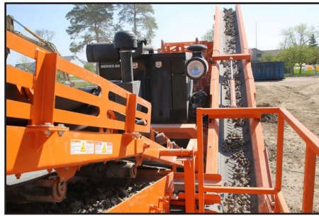
Top-deck retained material is returned to the crusher for further processing.
