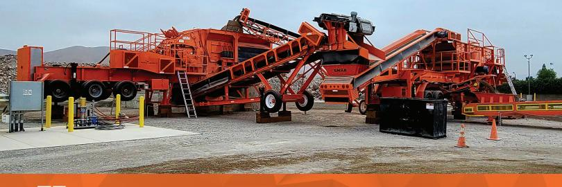
One of our most versatile systems utilizing a portable impactor plant and screening plant separately or combined to produce numerous spec products.
