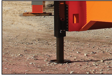
Hydraulic lift and leveling system enables quick set up and tear down.
