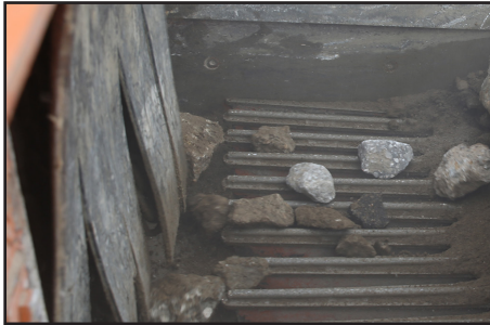
Features standard grizzly bypass chute and available cross-belt conveyor with flop gate.
