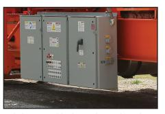
Includes removable electrical control panel featuring pre-wired receptacles for radial stackers.
