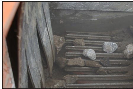
Screen products first before crushing, crush all products or crush with the grizzly product removed.
